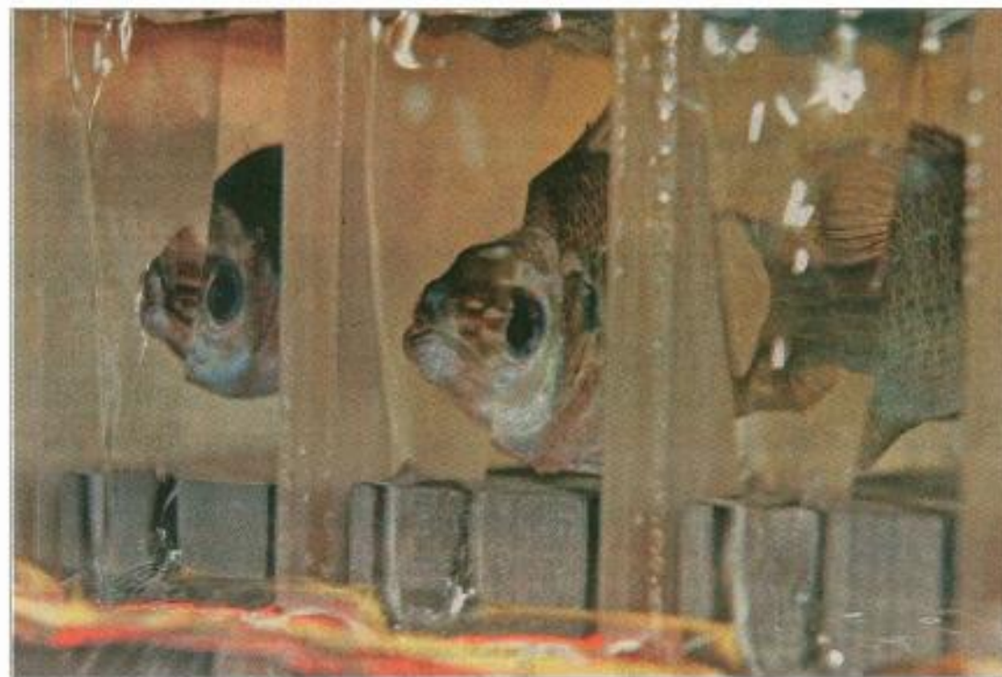
With passive electrodes above and below them, a team of bluegill fish swim in the individual chambers of a machine that constantly measures water quality. Agitated behavior in the fish is detected by a computer, which signals humans to take a closer look for toxins. After a two-week shift, the fish are transferred into an aquarium for some time off.
